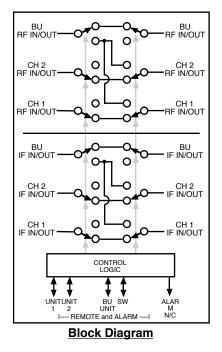
FIGURE 1.2 Model 2582-122 Switch Block Diagram
