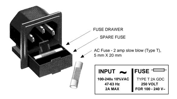
FIGURE 2.4 Fuse Location and Spare Fuse
