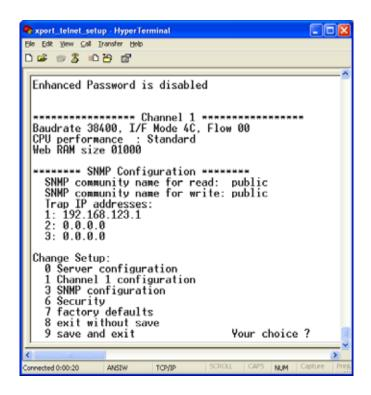
Figure 3.5: Device Server Configuration Menu
