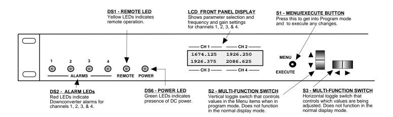
FIGURE 2.3 2416-x02l Front Panel Controls and Indicators
