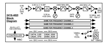
FIGURE 1.2 Model 2416-x02l Downconverter Block Diagram
