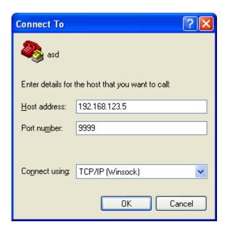
Figure 3.4: Telnet® Settings in Hyper Terminal
