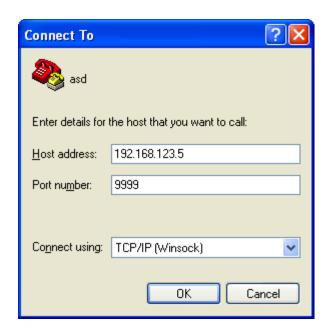
Figure 3.4: Telnet® Settings in Hyper Terminal
