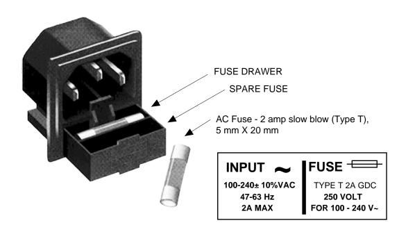
FIGURE 2.4 Fuse Location and Spare Fuse
