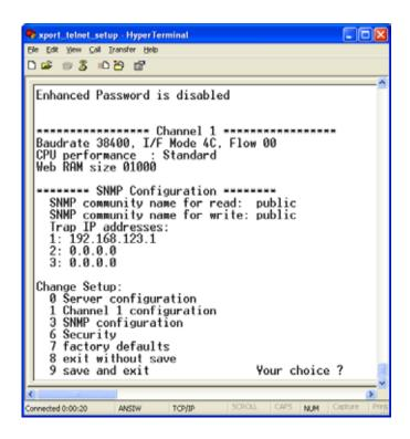
Figure 3.5: Device Server Configuration Menu
