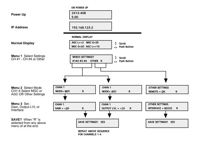
FIGURE 2.5 Model 2412-x08 Menu Display and Sequence
