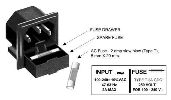
FIGURE 2.3 Fuse Location and Spare Fuse
