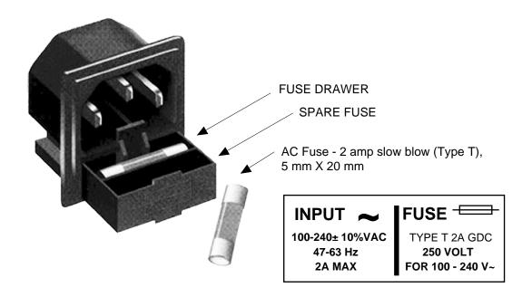
FIGURE 2.3 Fuse Location and Spare Fuse
