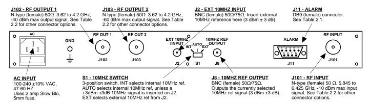
FIGURE 2.1 2116-6T4 Rear Panel I/O's
