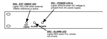
FIGURE 2.2 2116-35 Front Panel Controls and Indicators
