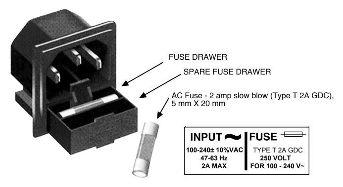
FIGURE 2.3 Fuse Location and Spare Fuse
