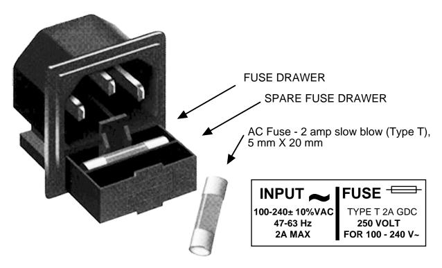
FIGURE 2.3 Fuse Location and Spare Fuse
