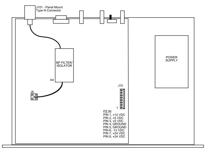
FIGURE 2.0 2116-34 Mechanical Assembly
