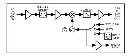
FIGURE 1.2 Model 2116-34 Downconverter Block Diagram
