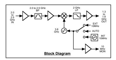
FIGURE 1.2 Model 2116-25 Downconverter Block Diagram
