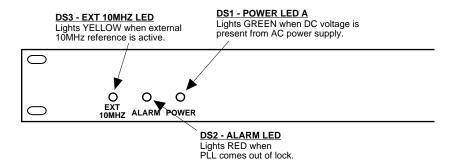
FIGURE 2.2 2116-25 Front Panel Controls and Indicators
