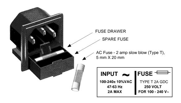
FIGURE 2.3 Fuse Location and Spare Fuse
