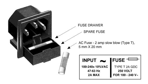
FIGURE 2.3 Fuse Location and Spare Fuse
