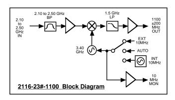
FIGURE 1.2 Model 2116-23#-1100 Downconverter Block Diagram
