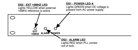
FIGURE 2.2 2116-222 Front Panel Controls and Indicators
