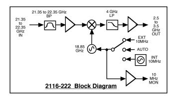
FIGURE 1.2 Model 2116-222 Downconverter Block Diagram
