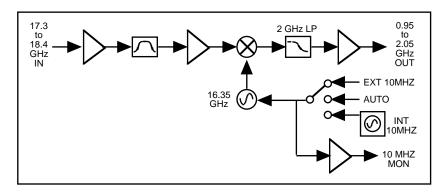
FIGURE 1.2 Model 2116-184 Downconverter Block Diagram
