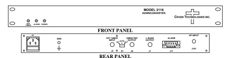
FIGURE 1.1 Model 2116-184 Front and Rear Panels
