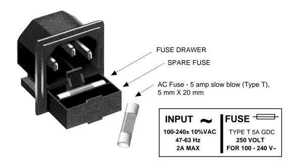
FIGURE 2.3 Fuse Location and Spare Fuse
