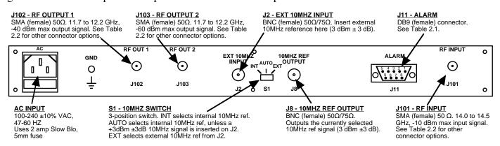
FIGURE 2.1 2116-14T12 Rear Panel I/O's
