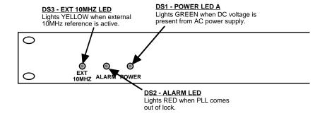
FIGURE 2.2 2116-14T12 Front Panel Controls and Indicators
