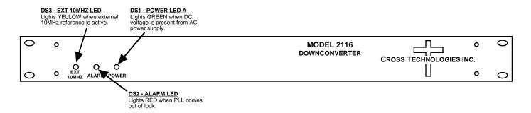
FIGURE 2.2 2116-140 Front Panel Controls and Indicators
