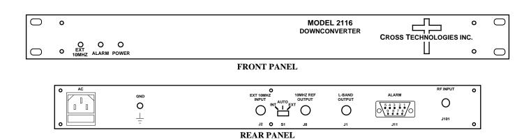
FIGURE 1.1 Front and Rear Panels
