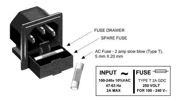
FIGURE 2.3 Fuse Location and Spare Fuse
