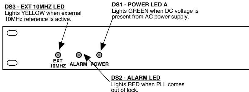
**FIGURE 2.2 2116-140T120 Front Panel Controls and Indicators**
