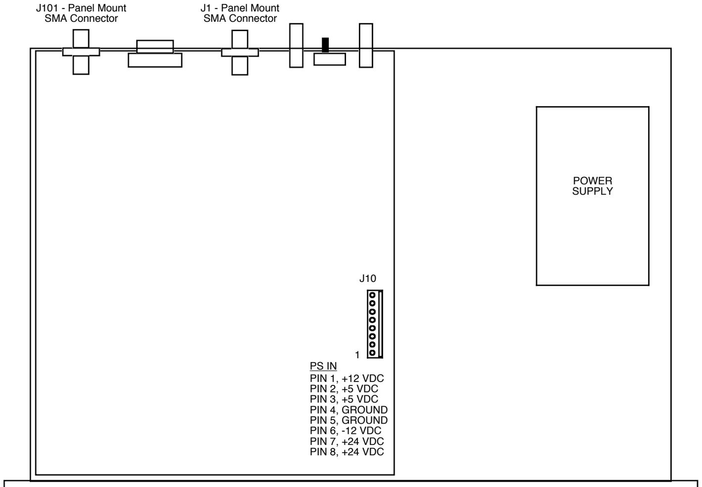
**FIGURE 2.0 2116-140T120 Mechanical Assembly**
