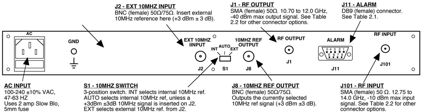
**FIGURE 2.1 2116-140T120 Rear Panel I/O's**
