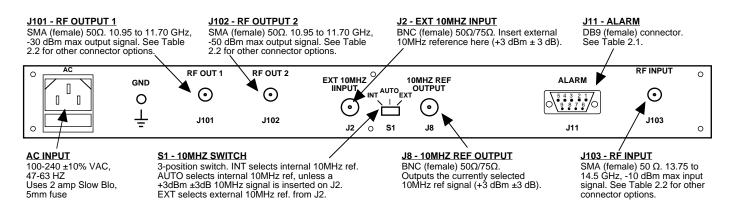
FIGURE 2.1 2116-13T11 Rear Panel I/O's
