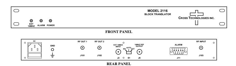
FIGURE 1.1 Front and Rear Panels
