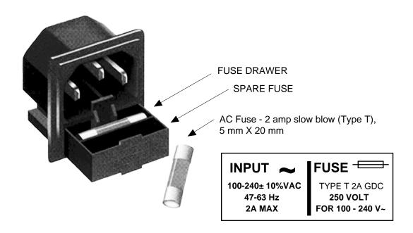
FIGURE 2.3 Fuse Location and Spare Fuse
