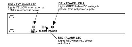
FIGURE 2.2 2116-13T11 Front Panel Controls and Indicators
