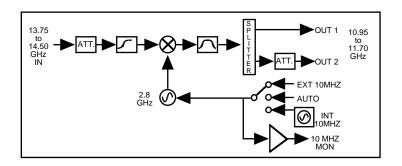
FIGURE 1.2 Block Diagram
