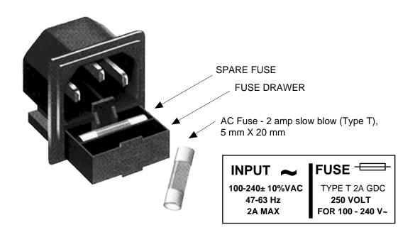
FIGURE 2.3 Fuse Location and Spare Fuse
