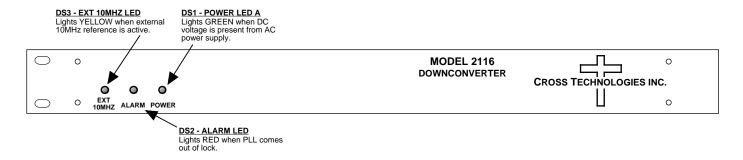
FIGURE 2.2 2116-139 Front Panel Controls and Indicators
