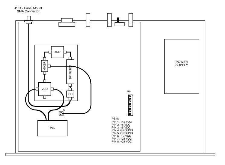
FIGURE 2.0 2116-137 Mechanical Assembly
