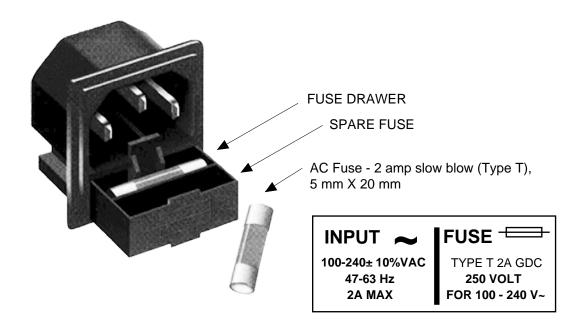
FIGURE 2.3 Fuse Location and Spare Fuse
