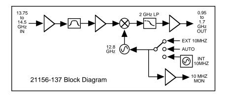
FIGURE 1.2 Model 2116-137 Downconverter Block Diagram
