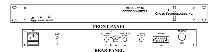
FIGURE 1.1 Model 2116-126 Front and Rear Panels
