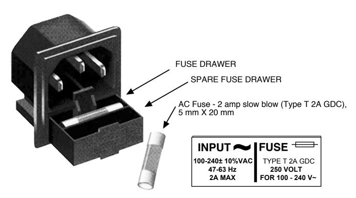
FIGURE 2.3 Fuse Location and Spare Fuse
