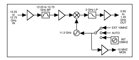
FIGURE 1.2 Model 2116-126 Downconverter Block Diagram
