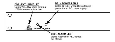
FIGURE 2.2 2116-126 Front Panel Controls and Indicators
