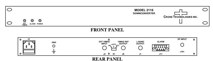
FIGURE 1.1 Model 2116-116 Front and Rear Panels
