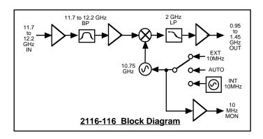
FIGURE 1.2 Model 2116-116 Downconverter Block Diagram
