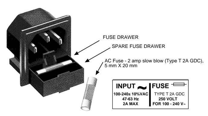
FIGURE 2.3 Fuse Location and Spare Fuse
