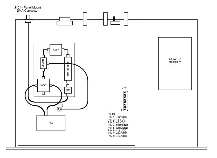
FIGURE 2.0 2116-116 Mechanical Assembly
