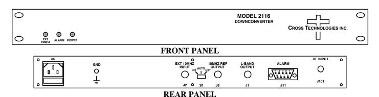
FIGURE 1.1 Model 2116-114 Front and Rear Panels
