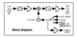
FIGURE 1.2 Model 2116-114 Downconverter Block Diagram
