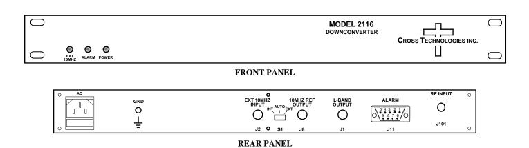
FIGURE 1.1 Model 2116-109 Front and Rear Panels
