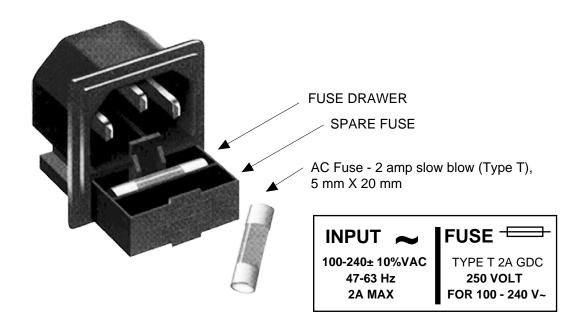
FIGURE 2.3 Fuse Location and Spare Fuse
