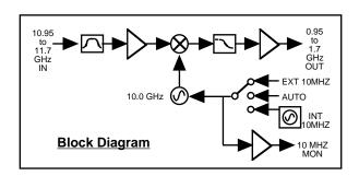
FIGURE 1.2 Model 2116-109 Downconverter Block Diagram
