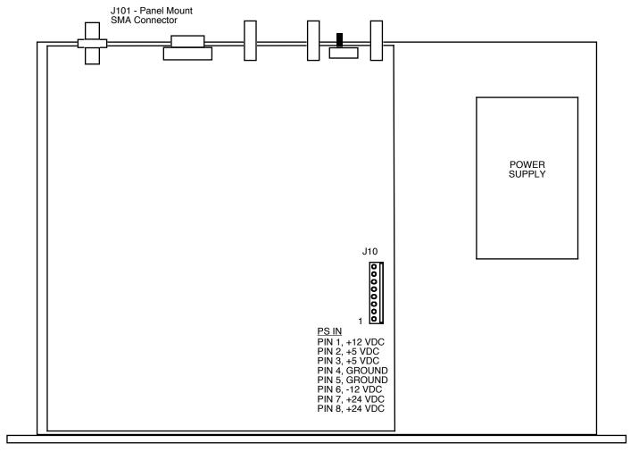
FIGURE 2.0 2116-105 Mechanical Assembly
