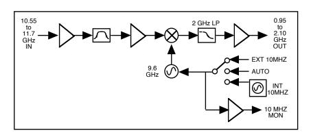
FIGURE 1.2 Model 2116-105 Downconverter Block Diagram
