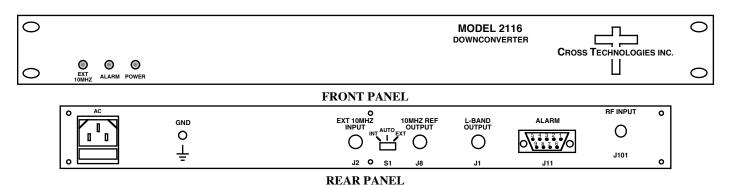
FIGURE 1.1 Model 2116-105 Front and Rear Panels
