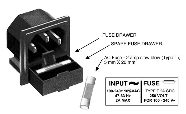
FIGURE 2.3 Fuse Location and Spare Fuse
