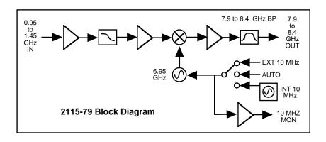
FIGURE 1.2 Block Diagram
