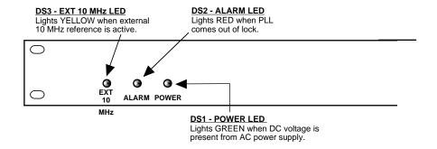
FIGURE 2.2 Front Panel Controls and Indicators
