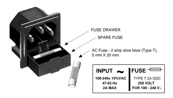
FIGURE 2.3 Fuse Location and Spare Fuse
