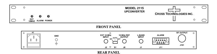
FIGURE 1.1 Front and Rear Panels
