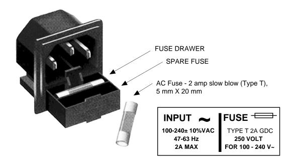
FIGURE 2.3 Fuse Location and Spare Fuse
