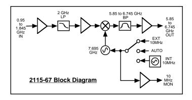
FIGURE 1.2 Block Diagram
