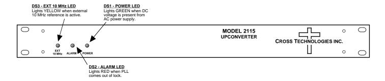
FIGURE 2.2 Front Panel Controls and Indicators
