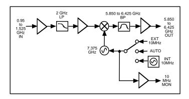
FIGURE 1.2 Model 2115-58 Upconverter Block Diagram
