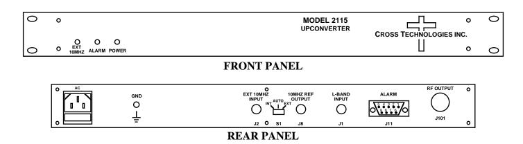
FIGURE 1.1 Model 2115-58 Front and Rear Panels
