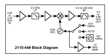
FIGURE 1.2 Block Diagram
