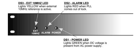
FIGURE 2.2 Front Panel Controls and Indicators
