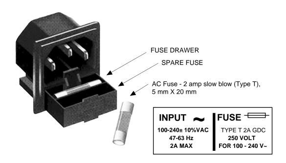
FIGURE 2.3 Fuse Location and Spare Fuse
