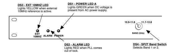
FIGURE 2.2 2115-21-109# Front Panel Controls and Indicators
