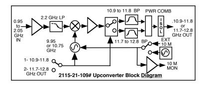
FIGURE 1.2 Model 2115-21-109# Upconverter Block Diagram
