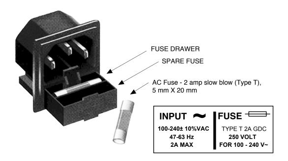
FIGURE 2.3 Fuse Location and Spare Fuse
