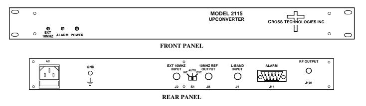
FIGURE 1.1 Model 2115-143 Front and Rear Panels
