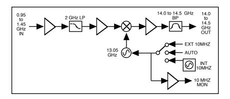
FIGURE 1.2 Model 2115-140 Upconverter Block Diagram
