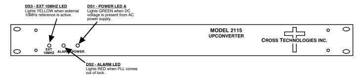
FIGURE 2.2 2115-140 Front Panel Controls and Indicators
