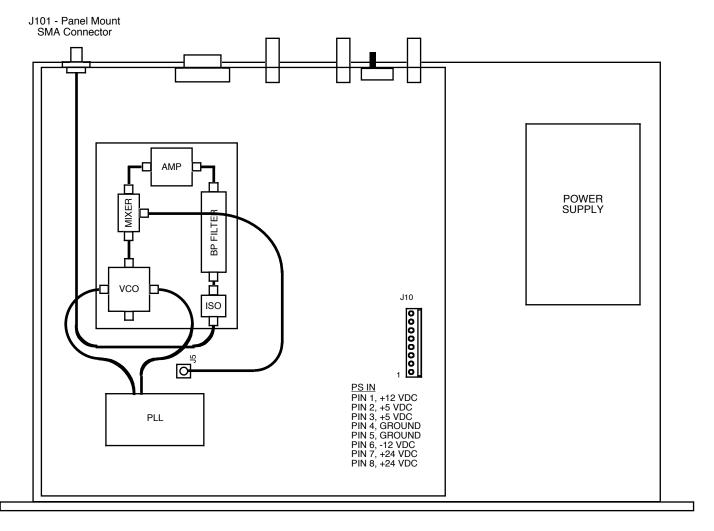
FIGURE 2.0 2115-140 Mechanical Assembly
