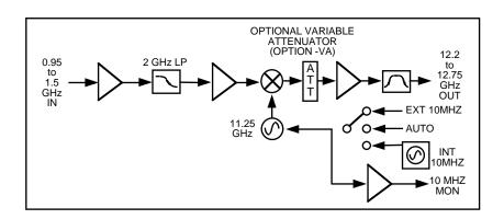
FIGURE 1.2 Model 2115-125 Upconverter Block Diagram
