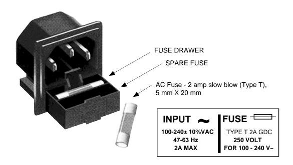
FIGURE 2.3 Fuse Location and Spare Fuse
