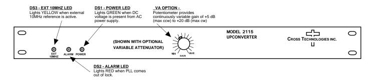
FIGURE 2.2 2115-125 Front Panel Controls and Indicators
