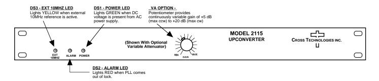
FIGURE 2.2 2115-109 Front Panel Controls and Indicators
