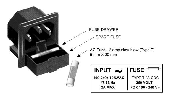
FIGURE 2.3 Fuse Location and Spare Fuse
