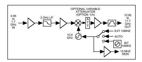
FIGURE 1.2 Model 2115-109 Upconverter Block Diagram
