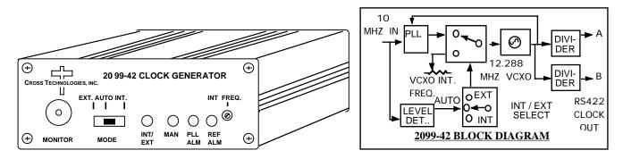
FIGURE 1.1 2099-42 Clock Generator Block Diagram and Front Panel
