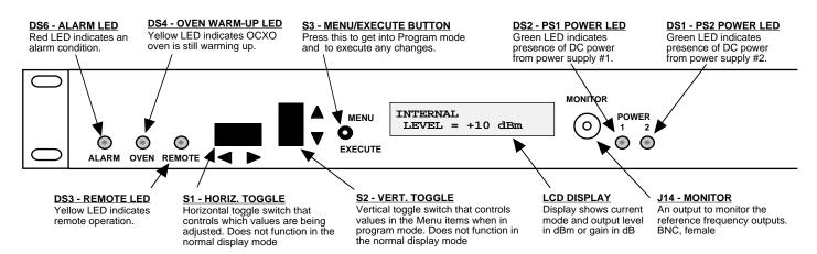
FIGURE 2.2 2099-25xx Front Panel Controls and Indicators
