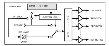
FIGURE 1.2 Model 2099-25xx 10MHz Frequency Source Block Diagram
