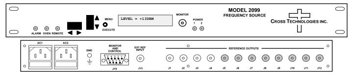
FIGURE 1.1 Model 2099-25xx Front and Rear Panels
