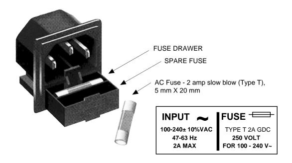
FIGURE 2.3 Fuse Location and Spare Fuse
