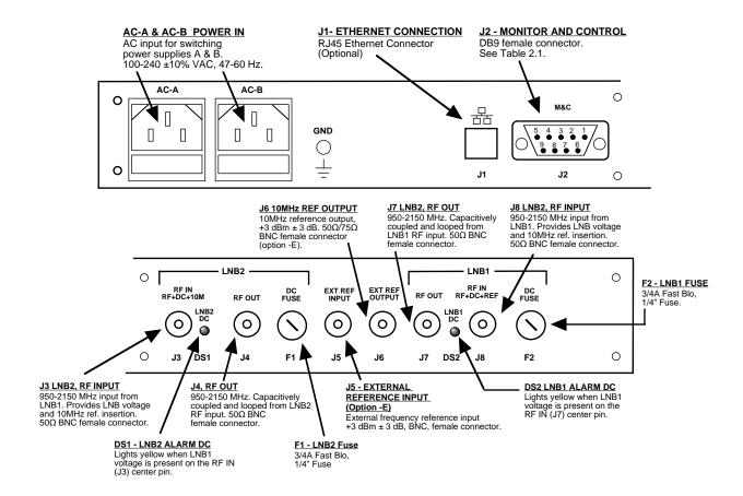
FIGURE 2.1 2099-24 Rear Panel Outputs
