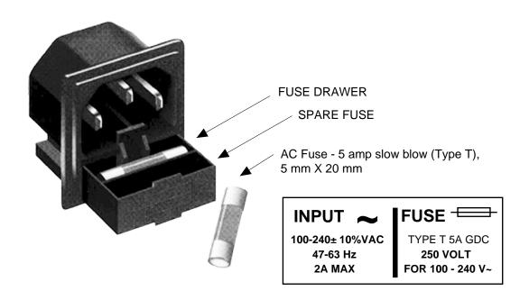
FIGURE 2.3 Fuse Location and Spare Fuse
