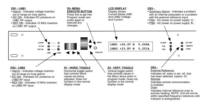
FIGURE 2.2 2099-24 Front Panel Controls and Indicators
