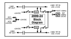
FIGURE 1.2 Model 2099-24 10MHz Source/Inserter Block Diagram
