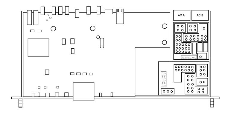
FIGURE 2.0 2099-24 10MHz Source/Inserter Mechanical Assembly
