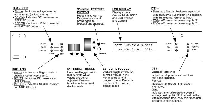
FIGURE 2.2 2099-2448 Front Panel Controls and Indicators
