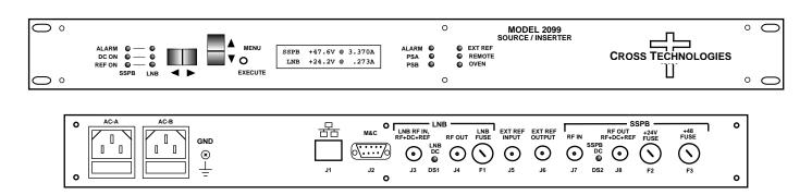
FIGURE 1.1 Model 2099-2448 Front and Rear Panels
