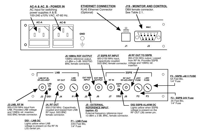
FIGURE 2.1 2099-2448 Rear Panel Outputs
