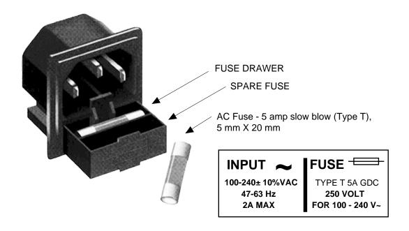
FIGURE 2.3 Fuse Location and Spare Fuse
