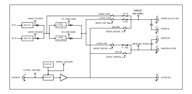
FIGURE 1.2 Model 2099-2448 10MHz Source/Inserter Block Diagram
