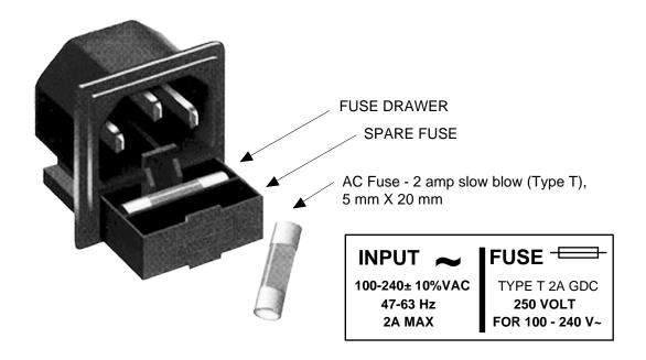
FIGURE 2.3 Fuse Location and Spare Fuse
