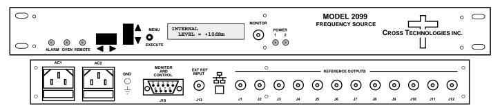
FIGURE 1.1 Model 2099-10xx Front and Rear Panels
