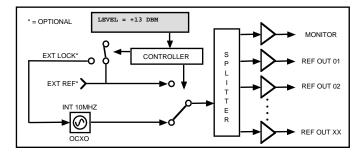
FIGURE 1.2 Model 2099-10xx 10MHz Frequency Source Block Diagram
