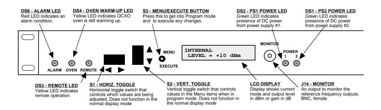
FIGURE 2.2 2099-10xx Front Panel Controls and Indicators
