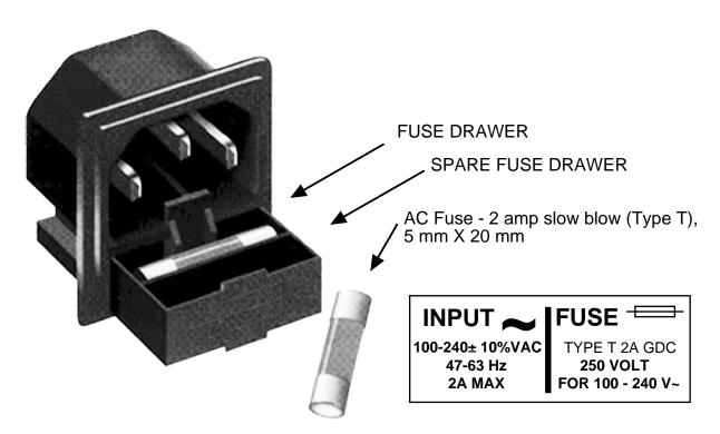
FIGURE 2.3 Fuse Location and Spare Fuse
