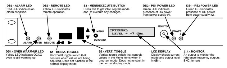
FIGURE 2.2 Front Panel Controls and Indicators
