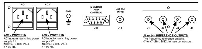
FIGURE 2.1 2099-10004 Rear Panel Outputs
