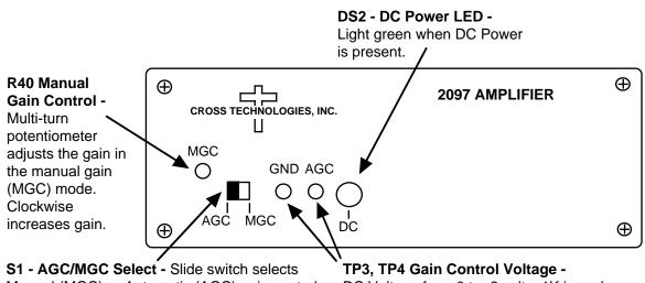
Manual (MGC) or Automatic (AGC) gain control. In (MGC) use R40 to adjust the gain.
