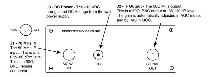
Figure 2.3 2097 Rear Panel Inputs and Outputs
