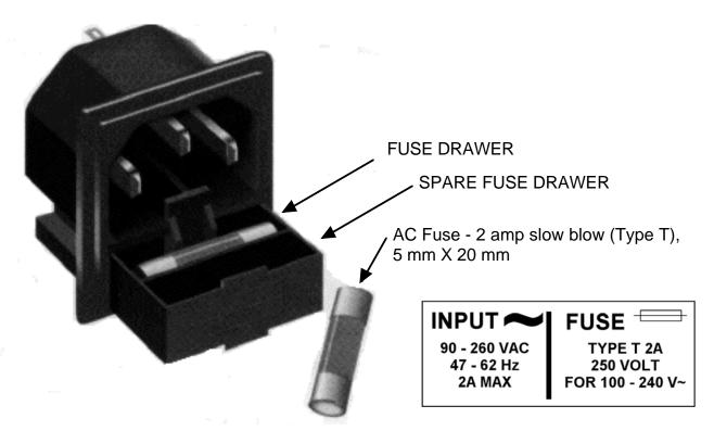
FIGURE 2.3 Fuse Location and Spare Fuse
