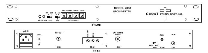
FIGURE 1.1 Model 2088-22 Front and Rear Panels
