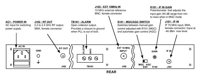
FIGURE 2.1 2088-22 Rear Panel I/Os and Level Control
