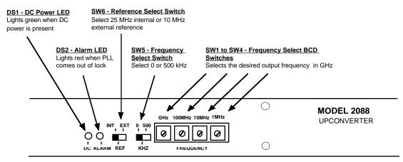
FIGURE 2.2 2088-22 Front Panel Controls and Indicators
