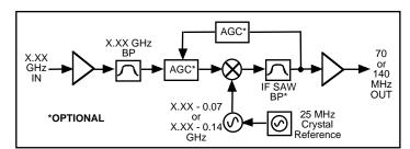
FIGURE 1.2 2087 Downconverter Block Diagram
