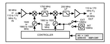
FIGURE 1.2 Model 2083-914A Translator Block Diagram
