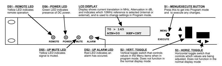
FIGURE 2.2 2083-914A Front Panel Controls and Indicators
