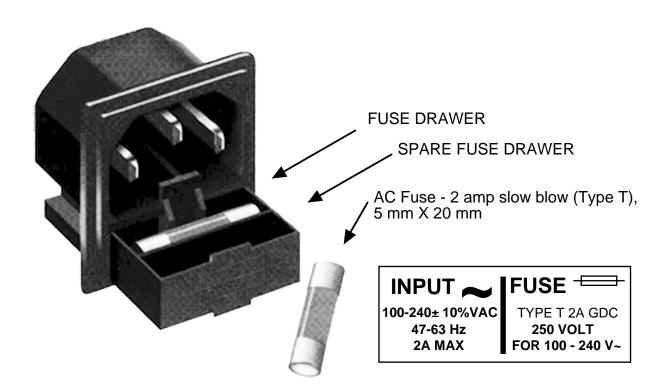
FIGURE 2.3 Fuse Location and Spare Fuse
