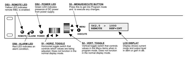
FIGURE 2.2 2083-910 Front Panel Controls and Indicators
