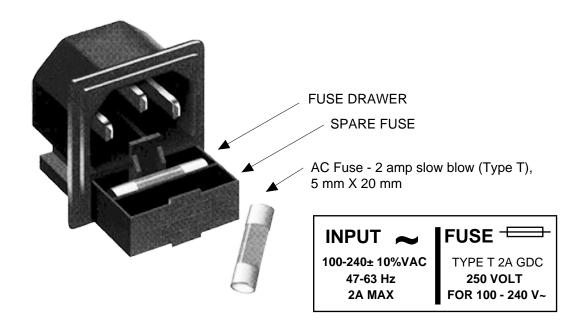
FIGURE 2.3 Fuse Location and Spare Fuse
