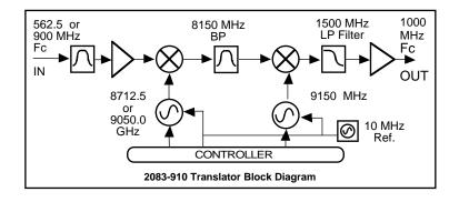
FIGURE 1.2 2083-910 Block Diagram
