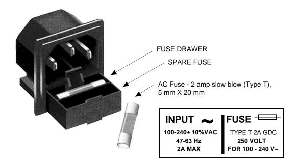
FIGURE 2.3 Fuse Location and Spare Fuse
