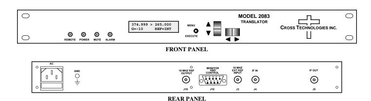
FIGURE 1.1 Model 2083-43 Front and Rear Panels
