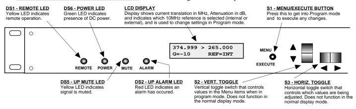
FIGURE 2.2 2083-43 Front Panel Controls and Indicators
