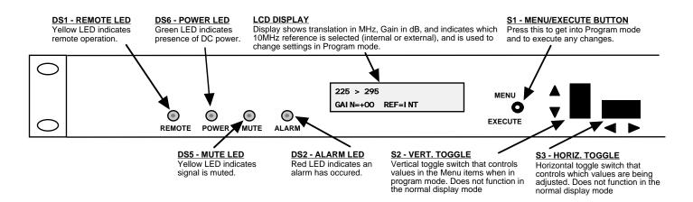
FIGURE 2.2 2083-22 Front Panel Controls and Indicators
