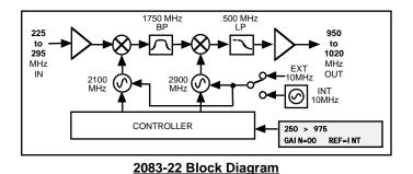
FIGURE 1.2 Model 2083-22 Translator Block Diagram
