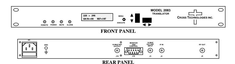
FIGURE 1.1 Model 2083-22 Front and Rear Panels
