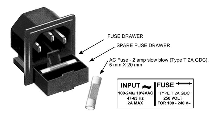
FIGURE 2.3 Fuse Location and Spare Fuse
