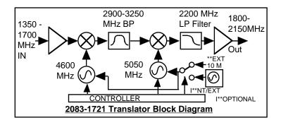
FIGURE 1.2 Block Diagram
