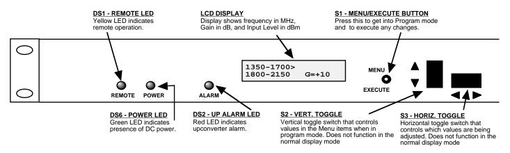
FIGURE 2.2 2083-1721 Front Panel Controls and Indicators
