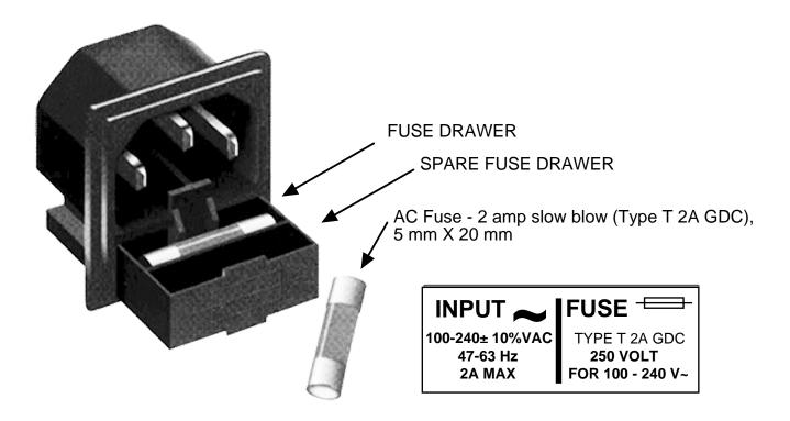
FIGURE 2.3 Fuse Location and Spare Fuse
