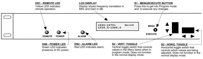
FIGURE 2.2 2083-1615 Front Panel Controls and Indicators
