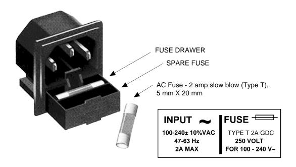
FIGURE 2.3 Fuse Location and Spare Fuse
