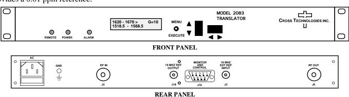
FIGURE 1.1 2083-1615 Front and Rear Panels
