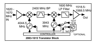
FIGURE 1.2 2083-1615 Block Diagram
