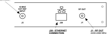
RJ45 Ethernet Connector (Option W8, W18, W28) <u>J1 - RF OUT</u> 2240-2260 MHz output -30 to -50 dBm See Table 2.2.
