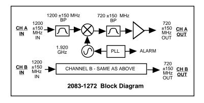
FIGURE 1.2 Model 2083-1272 Block Diagram
