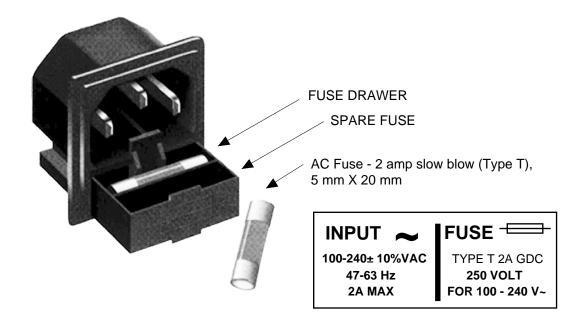
FIGURE 2.3 Fuse Location and Spare Fuse
