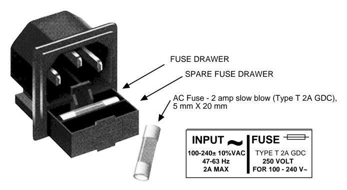
FIGURE 2.3 Fuse Location and Spare Fuse
