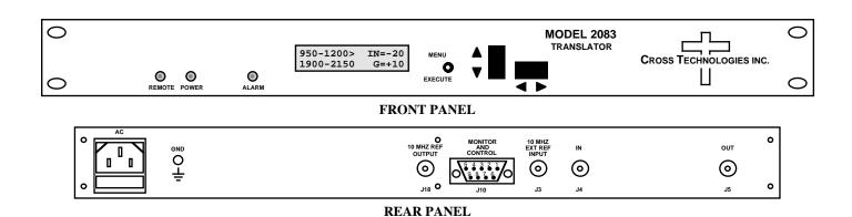
**FIGURE 1.1 Front and Rear Panels**
