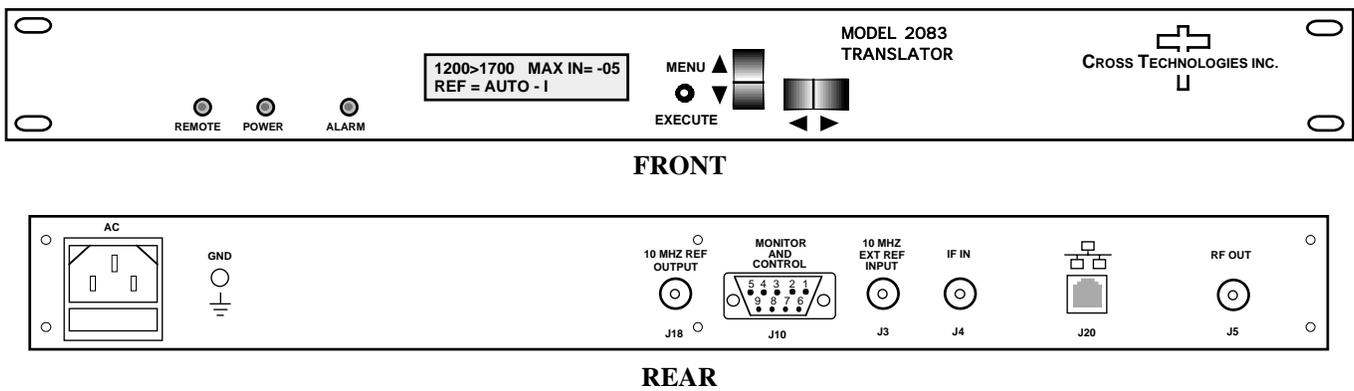
**FIGURE 1.1 Model 2083-0914 Front and Rear Panels**
