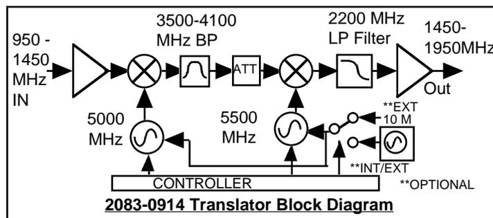
**FIGURE 1.2 Model 2083-0914 Translator Block Diagram**
